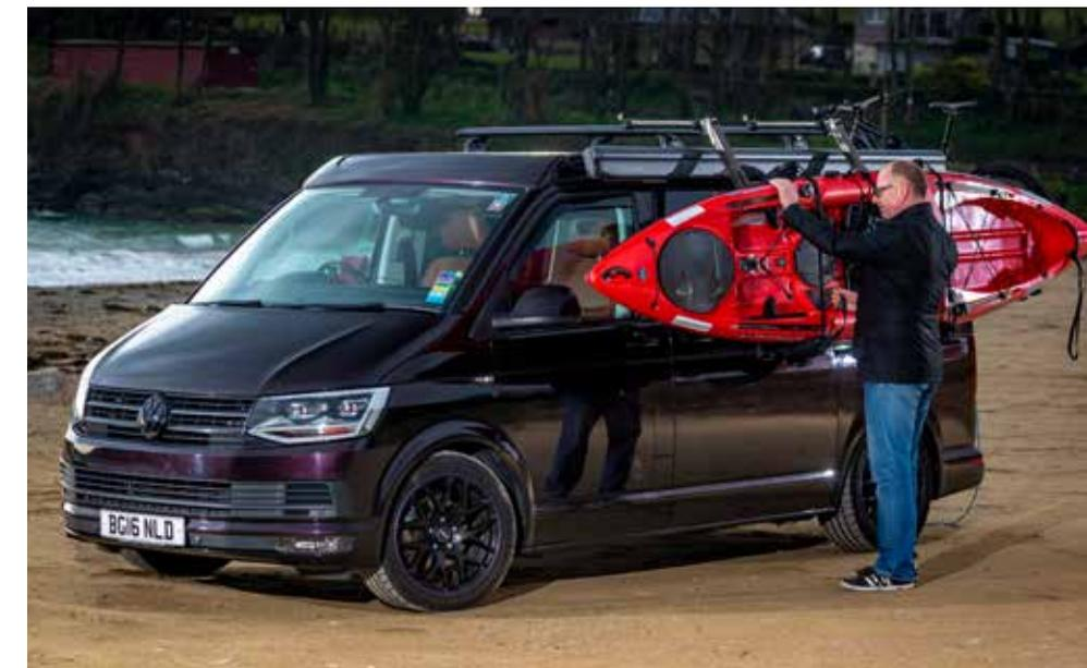
▲ Gas assisted struts on the Thule Hullavator kit makes loading the kayak a one-person job
